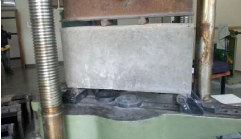
Figure1. Experimental Setup for Testing of Beams.
